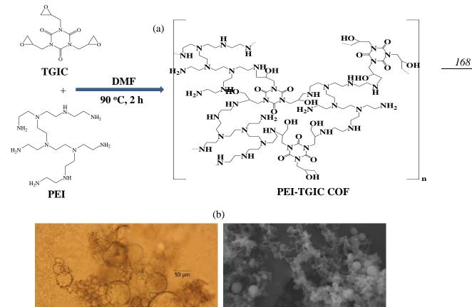
It was clearly seen from optic microscope and SEM images of PEI-TGIC COFs, the COFs are spherical shape with poly dispersed size ranges. The optic microscope images of PEI-TGIC COFs were taken from the aqueous solution of COFs, and it was seen that, the sizes of
