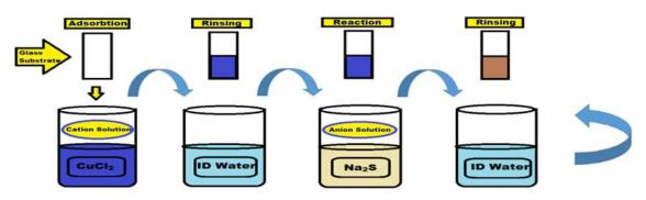
Figure 1. Schematic representation of SILAR method.
