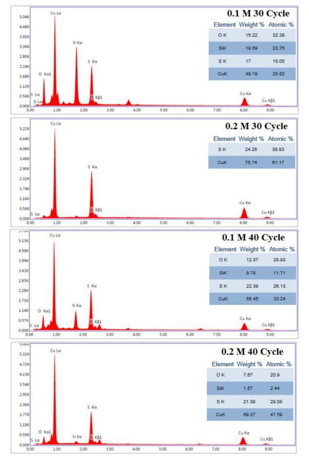
Figure 5. EDX images of 0.1 M and 0.2 M CuS thin films grown at 30 and 40 cycles.
