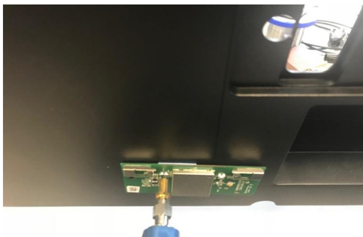
Fig. 8. Wi-Fi module placed on Plastic Surface
