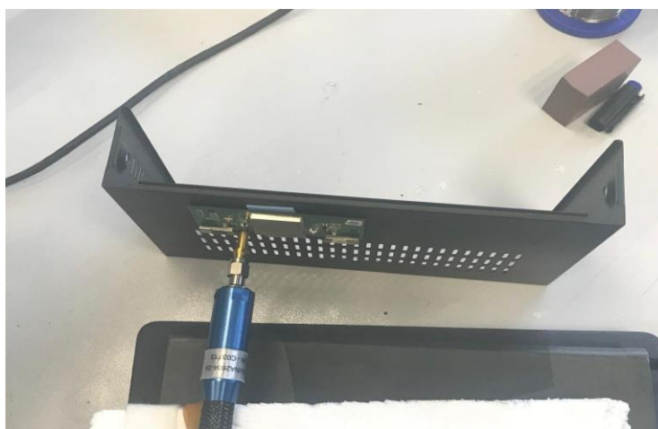
Fig. 7. Wi-Fi module placed on Metal Surface
