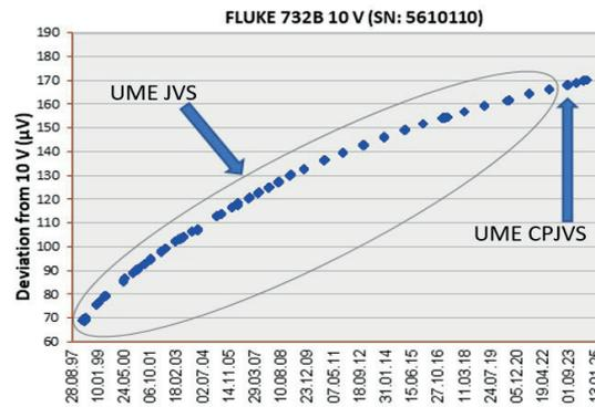
**Figure 5.** Long-term Drift of the DC Standard
