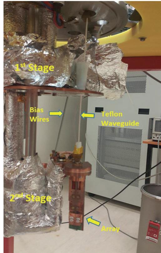
Figure 2. Array and Wiring Inside the Cryocooler
