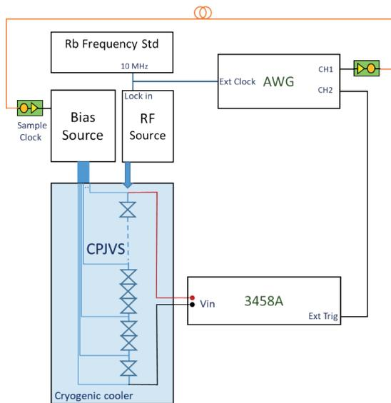
**Figure 6.** System for Testing Digitizer Using UME CPJVS
