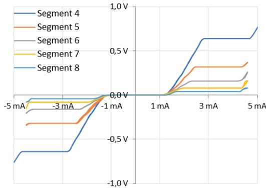
**Figure 4.** I-V characteristics of Segments 4-8
