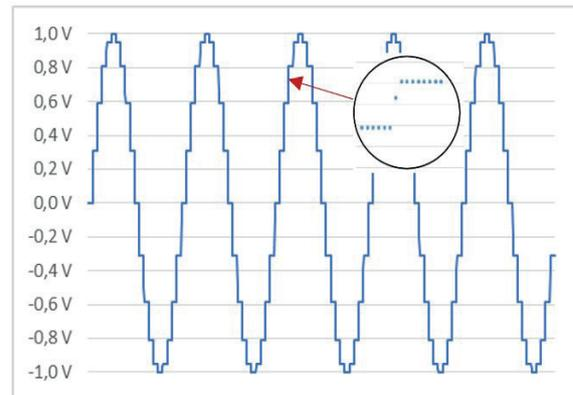
**Figure 7.** UME CPJVS Step-Approximated Sine Wave Measured by Digitizer
