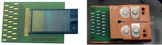
Figure 1. Josephson Array (a) with Thermal Interface (b)
